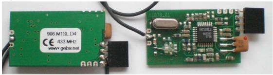
The position and direction of the RC receiver module depends on the type of control. Please see the red marks for the positioning and the picture aside for the direction of the receiver module.
